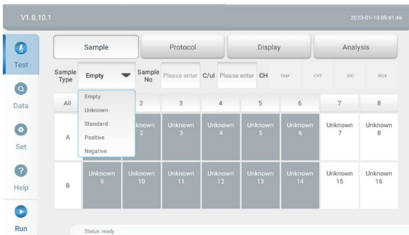
Click <Sample No> or <C/μL> to enter the sample ID or sample system, as shown in the figure below:
