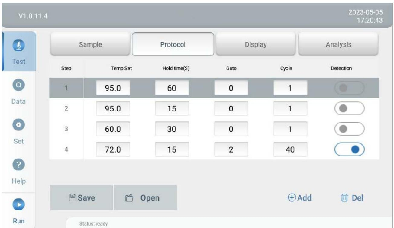
**NOTE: In the Detection column, signal collection must be turned on in the collection step.**
