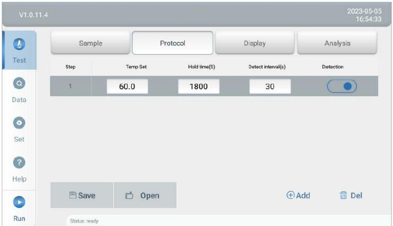
The constant temperature equipment needs to set the temperature, total time and detection interval, and pay attention to strobe the detection switch while setting the detection interval step.
