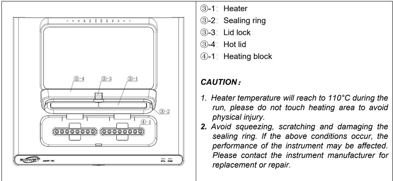
**Hot lid:** The heater is located inside of the hot lid to prevent the evaporation of reagent from condensing on the reaction tube. Before the experiment, the hot lid must be pressed in place. When the experiment is completed, press the door button to open the hot lid.
